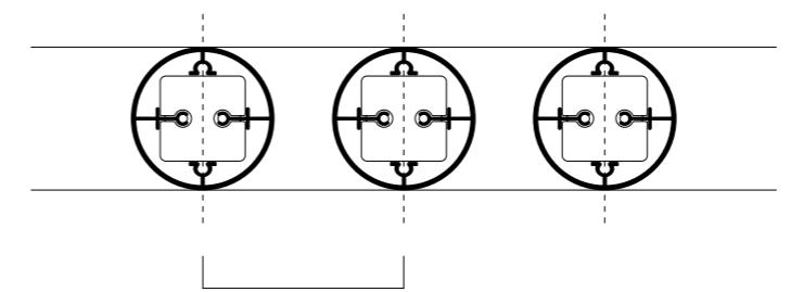
Fixing plate minimum width = stripe width
