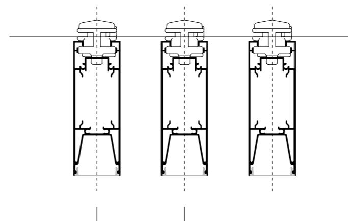
Free pitch defined during project. Minimum interaxial pitch 65 mm, 30 mm spacing.
