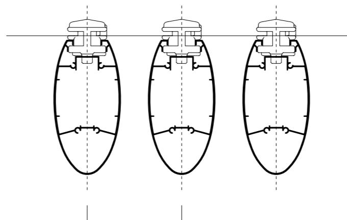
Free pitch defined during project. Minimum interaxial pitch 70 mm, 20 mm spacing.
