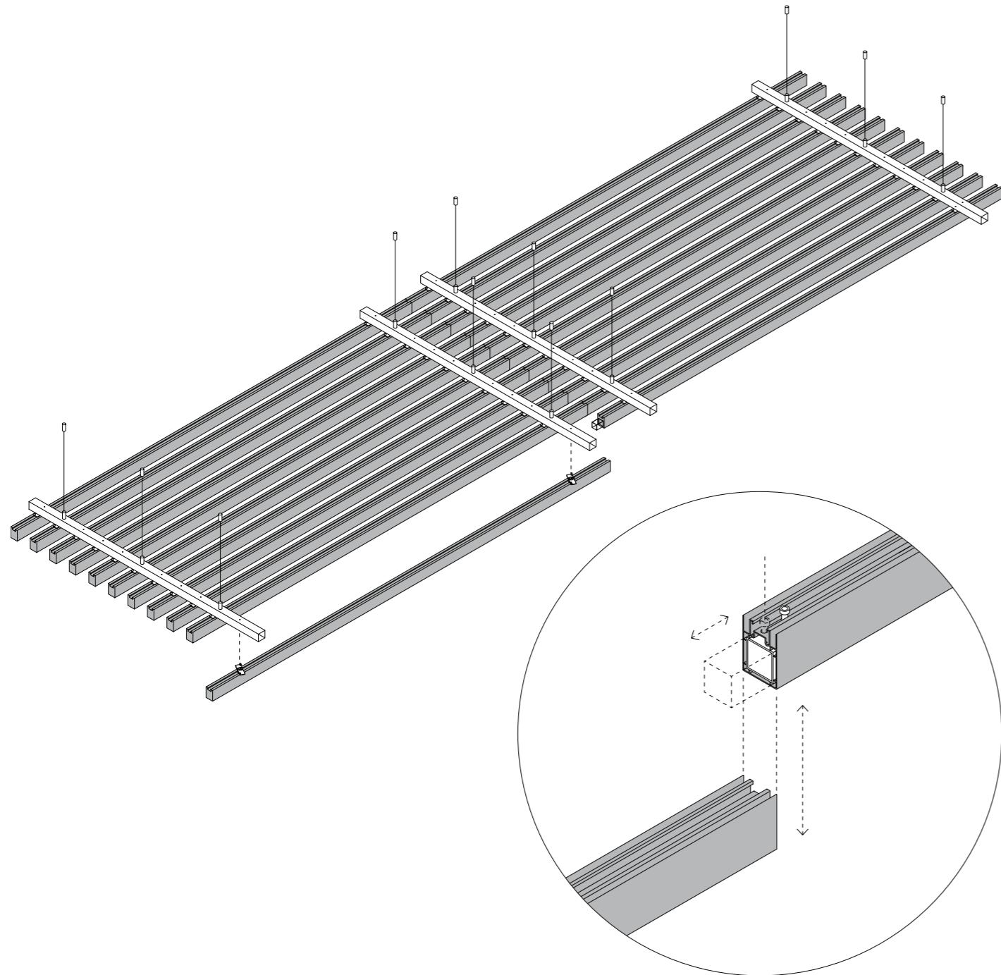
We've developed closing caps as accessories to be used in specific instances. The top closing cap is mandatory only when lighting slats are involved, while the rear closing cap is employed whenever slats are visible from both sides. Both caps benefit from a seamless, invisible application to the slat.
