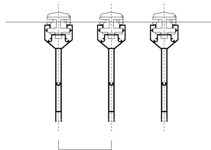
Free pitch defined during project. Minimum interaxial pitch 65 mm, 30 mm spacing.
