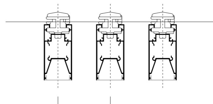
Free pitch defined during project. Minimum interaxial pitch 65 mm, 30 mm spacing.
