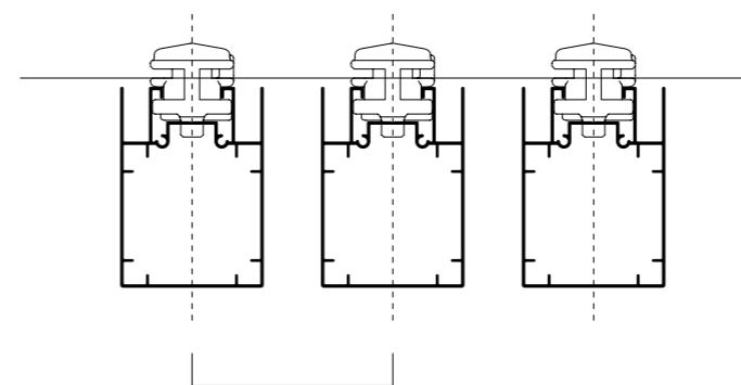
Free pitch defined during project. Minimum interaxial pitch 70 mm, 20 mm spacing.
