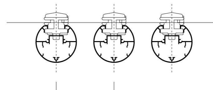
Free pitch defined during project. Minimum interaxial pitch 70 mm, 20 mm spacing.
