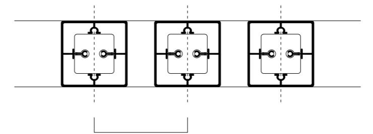
Free pitch defined during project. Minimum interaxial pitch 70 mm, 20 mm spacing.
